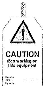
Fig.4A: 'Caution, men working on this equipment' tag
